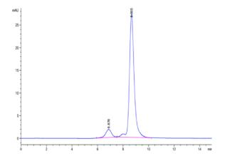
The purity of Cynomolgus IL-17A is greater than 90% as determined by SEC-HPLC.
